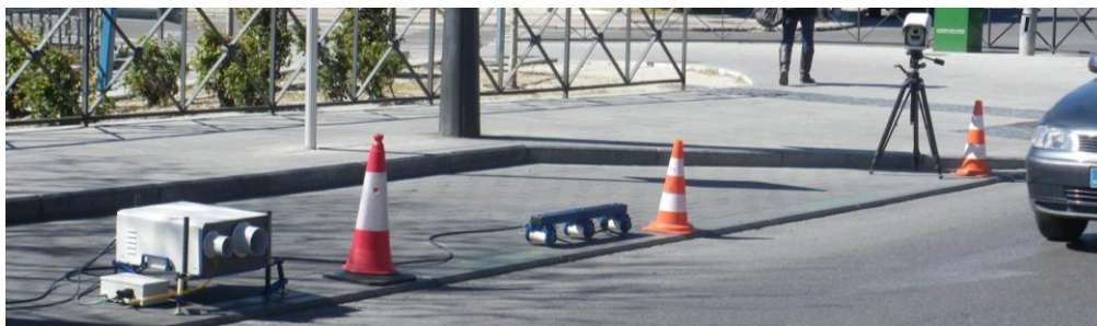
RSD Deployment (from left to right): IR/UV source/detector, speed/acceleration sensor, digital camera
